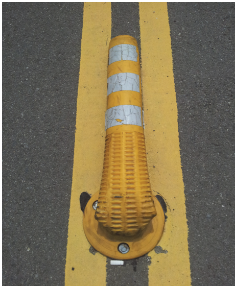
(c)受撞後完全傾倒不起
