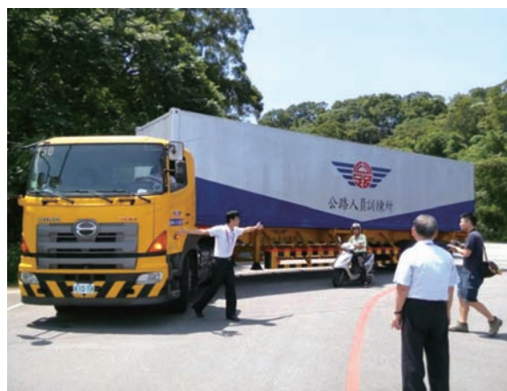
Difference of Radius Between Inner Wheels
