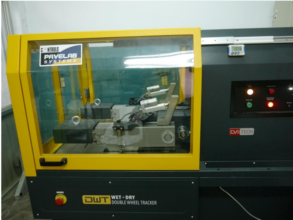
Hamburg Wheel Tracking Test (Photo taken by DGH)
