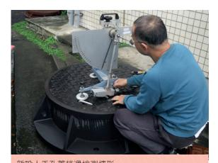
新設人手孔蓋抗滑檢測情形。 The situation of anti-slip detection of the newly set manhole cover.
